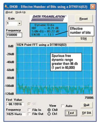
Figure 16. This graph shows the outstanding quality of the DT9816-A for all error sources ... effective number of bits greater than 13.1 from all sources. Note the absence of harmonic content and digital switching noise across the full spectrum.
