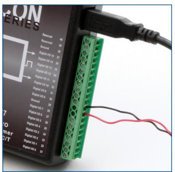
Figure 7. Connect sensors directly to the screw terminal of the module. Screw terminals can accept AWG 26 to AWG 16 size wire.
