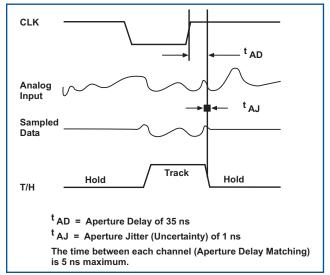
Figure 15. The A/D design of the DT9816 modules feature built-in accuracy. A maximum aperture delay of 35 ns (the time that it takes the A/D to switch from track to hold mode) is well matched at 5 ns across all six track-and-hold circuits, virtually eliminating the channel-to-channel skew that is associated with multiplexed inputs. A maximum aperture uncertainty of 1 ns (the jitter or variance in aperture delay), virtually eliminates phase noise in your data.
