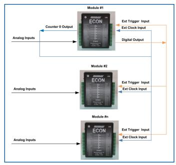
Figure 17. You can synchronize the analog I/O operations of multiple modules by connecting them together.
