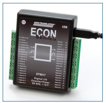
Figure 6. Connect to a host computer using the standard USB 1.1 or 2.0 plug-in connector on the ECONseries module. The USB connector provides power to the module, eliminating the need for an external power supply, while providing complete enumeration for all data flow.
