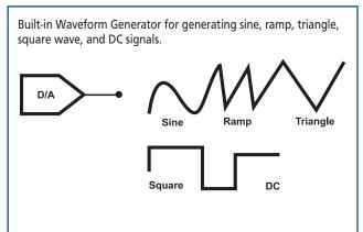
Figure 12. The DT9812-10V, DT9813-10V, and the DT9814-10V modules provide 2 waveform DACs for generating sine, ramp, triangle, square wave, and DC signals.
